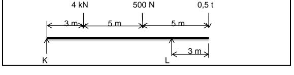
2.2.1 Ignore the weight of the beam and calculate the reactions of the supports of the beam by taking moments in kN about each support, namely K and L.
